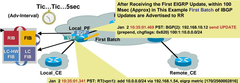
When first batch is received on RR, routes are immediately sent to the remote PE
