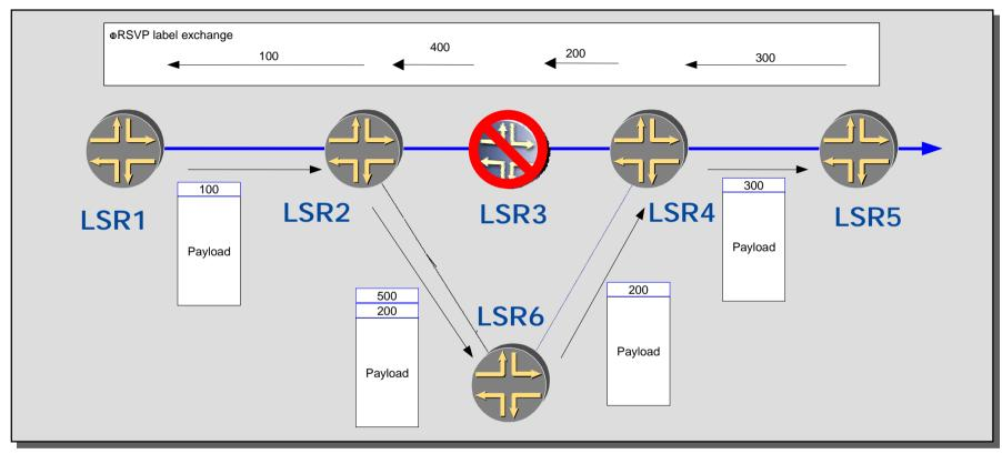
Each LSR detects that an interface has gone down and reroutes all the Protected LSPs traversing the interface via the Bypass LSP
